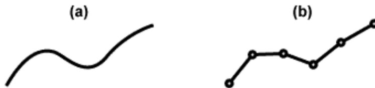
FIG. 2.1. (a) A continuous boundary. (b) A discrete representation of the continuous boundary. In (b), nodes are indicated by the circles and elements are indicated by the straight lines.
